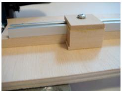
Finally I made an auto hold down from a strip of 1/4" wide spring steel positioned such that it is compressed when the saw is pressed down. I also had to buy a much more of this spring steel than I will ever use but it also was cheap. I bolted the spring steel to the base with 2-56 flat head screws.
