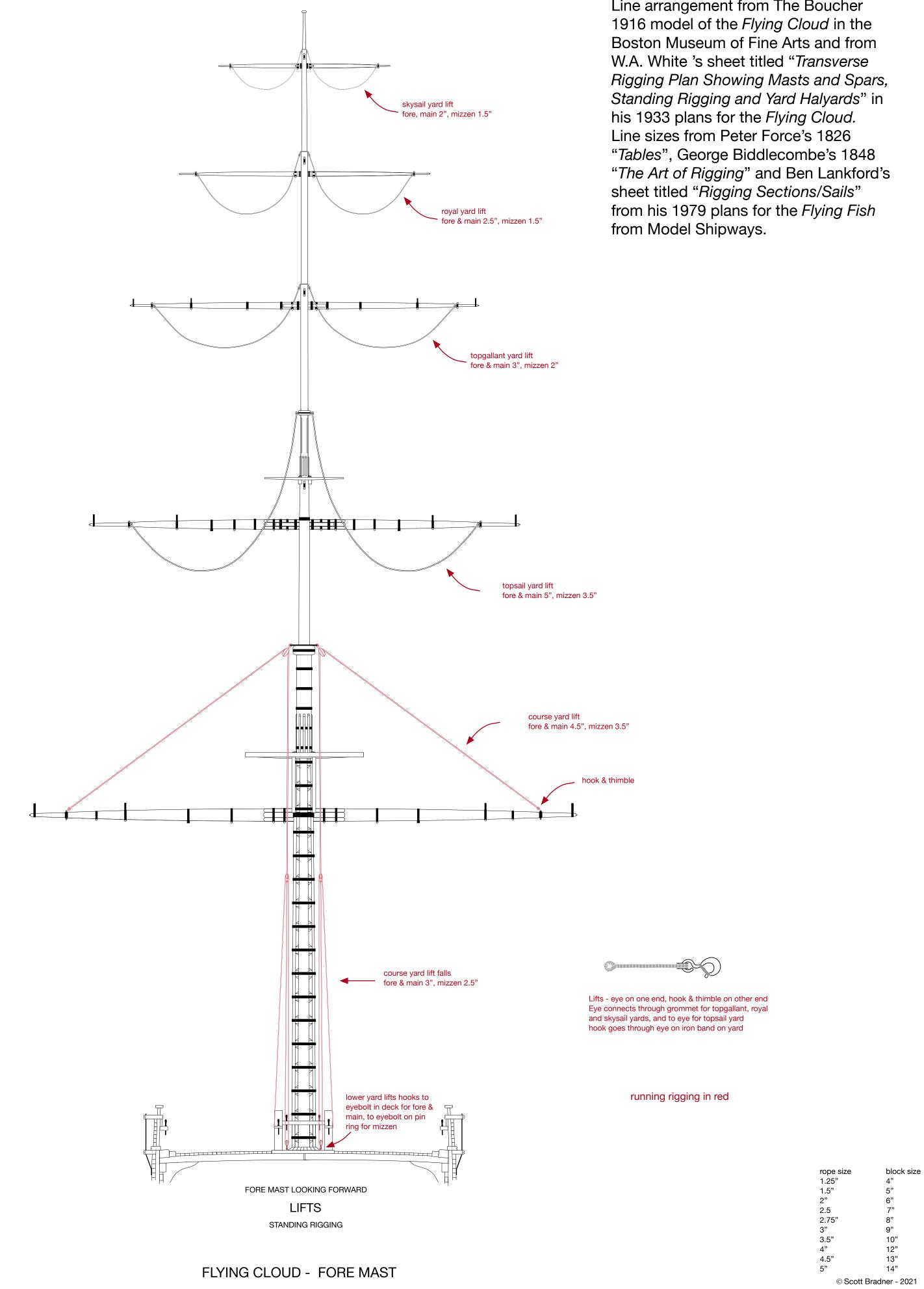
Line arrangement from The Boucher "The Art of Rigging" and Ben Lankford's
