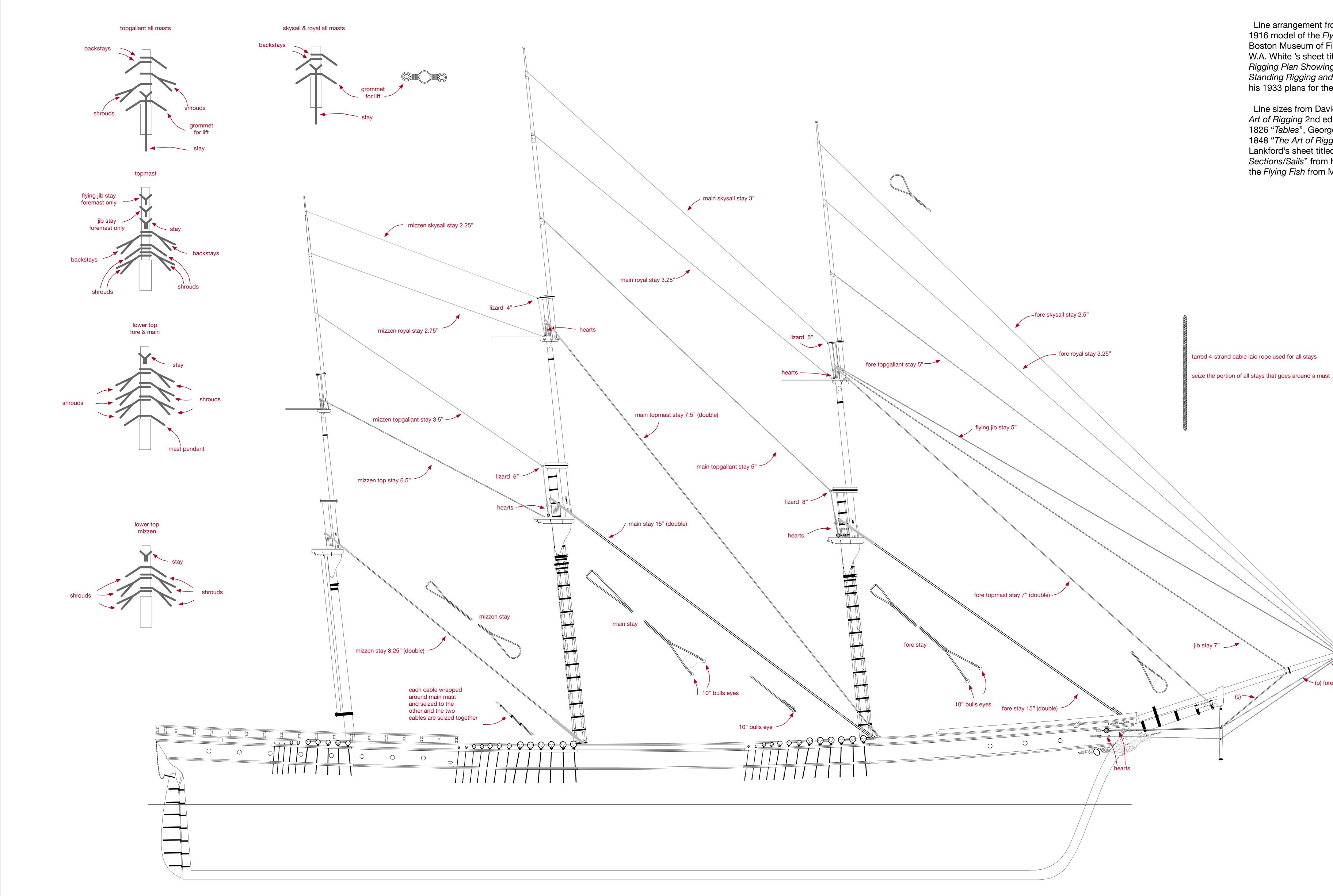
Line arrangement from The Boucher 1916 model of the Flying Cloud in the Boston Museum of Fine Arts and from W.A. White 's sheet titled "Transverse Rigging Plan Showing Masts and Spars, Standing Rigging and Yard Halyards" in his 1933 plans for the Flying Cloud.
